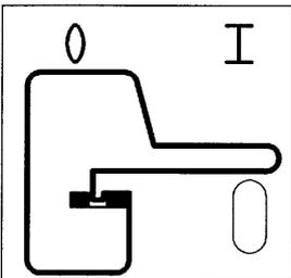
A spring presses the gear shift lever into a locking recess. In this position the band brake is slightly loosened and does not have any braking action during the wind-up.
