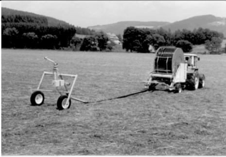
Lower the cart as described in Operating mode I, chapter "Lowering the cart" and anchor it slightly. Now drive over the field with the machine.
