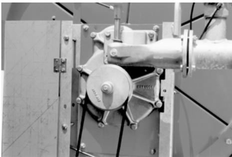
TX20 full-flow turbine is a specifically designed turbine with large cross sections and minimum pressure loss. Therefore it can reach high retraction speeds also at very low flow rate. It features a highly flow-promoting design and is mounted directly on the reel shaft. The turbine provides the energy needed for PE-pipe retraction. Speed is taken directly off the impeller shaft and transmitted over a two-stage (three-stage) V-belt drive to the change-speed gearbox.
