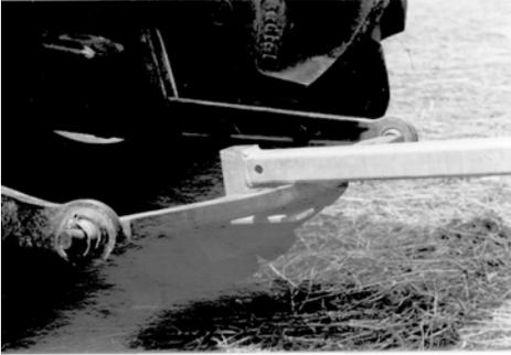
When the full operating pressure has been reached and only clear water is discharged at the sprinkler's nozzle in a full jet without air bubbles, push the gear shift lever to the "PE-pipe retraction" position.
