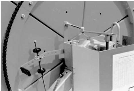
... and the regulating rods which actuate the regulating flap located directly on the turbine.
