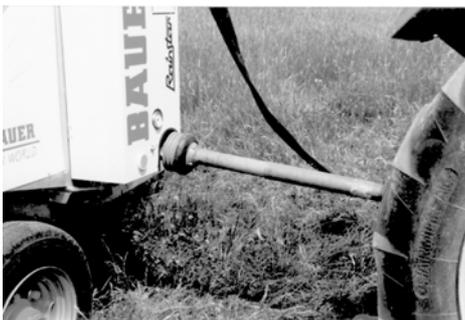
If required, you can rewind the PE-pipe with the tractor and a PTO shaft. Move the gear shift lever to zero position. A spring presses the gear shift lever into the locking recess. In this position the band brake is released. This gear shift lever position serves also for PE-pipe pull-off.
