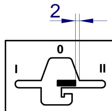
If the spacing is smaller than 1 mm or large than 3 mm, the difference must be split up equally on both sides!
