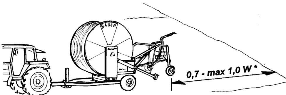
Drive the RAINSTAR into the field allowing for the sprinkler's distance of throw.
