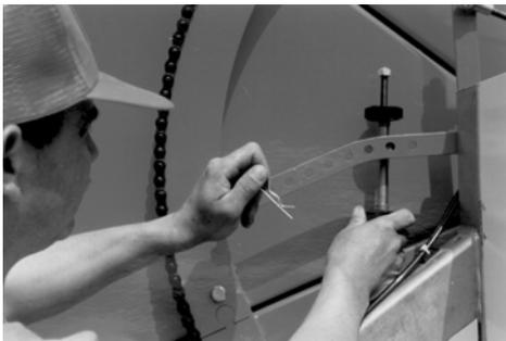
Varying soil conditions and low flow rates may cause uneven retraction speeds in spite of the layering mechanism. If retraction speeds up or slows down, the regulating rod must therefore be hooked up in the next suitable hole.
