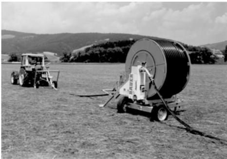
The standard wheel cart or the asymmetric wheel cart need not be hoisted (therefore 1 draw-out hook is sufficient).
