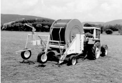
During transport the reel should be turned into the driving direction and secured with the lock bolt. Cart, jack, and both rear support legs must be lifted or withdrawn. For lateral PE-pipe pull-off, set up the RAINSTAR on the headland at right angles to the selected irrigation strip and detach it from the tractor.
