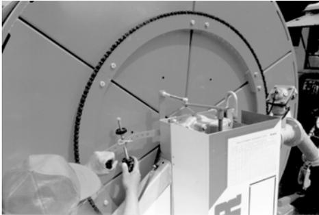
The retraction speed is infinitely variable with the speed regulating lever which is secured with the knurled nuts after the setting. It remains next to constant from the first to the last layer and on each individual layer. This is achieved by readjustment of the turbine speed through the speed compensation bar fitting closely on every PE-pipe layer during the run ...
