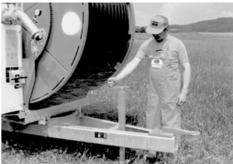
Adjust the undercarriage about level with the jack.
