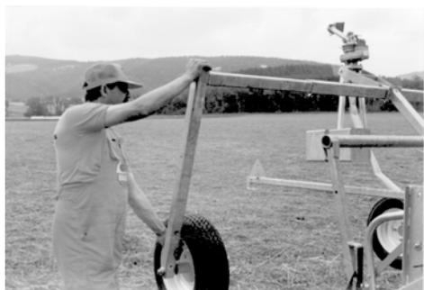
Set the required track width on high-rise cart and RAINSTAR undercarriage, depending on the existing type of crop.
