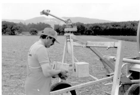
Place the appropriate number of balancing weights on the balancing pendulum of the cart. Two weights will do for nozzle diameters from 14 to 24 mm. For diameters larger than 24 mm two additional weights should be placed on the pendulum when the smallest track width setting is used.
