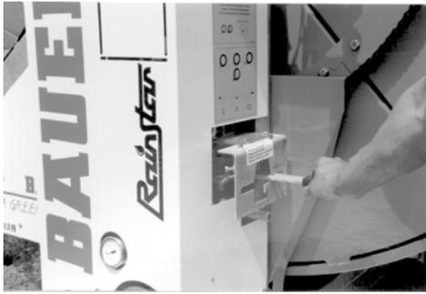
When the full operating pressure has been reached and clear water is discharged at the sprinkler's nozzle in a full jet without air bubbles, push the gear shift lever to the "PE-pipe retraction" position.
