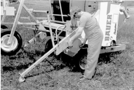
Drive the supports into the ground with the detachable hand wheel ...
