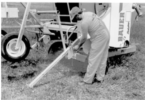
Move gear shift lever into the "PE-pipe pull-off" position. A spring presses the lever up and locks it.
