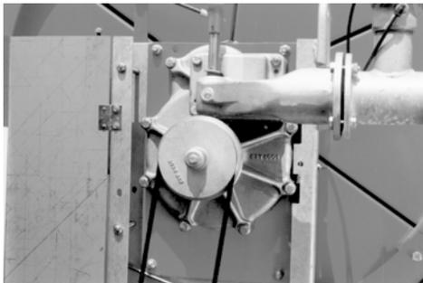
The TX20 full-flow turbine is a specifically designed turbine model with large cross sections and minimum pressure loss. Therefore it is also suited for high retraction speeds at very low flow rates. This turbine features a highly flow-promoting design and is mounted directly on the reel shaft. It provides the energy needed for PE-pipe retraction. The turbine speed is taken directly off the impeller shaft and transmitted over a V-belt drive to BAUER change-speed gearbox.
