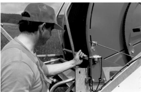
Before starting up with water again the hand lever of the three-way cock must be shifted to the START position (downward) - the shut-off valve is relieved and opens.
