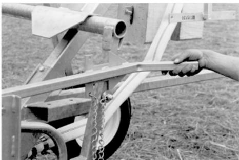
Disengage the mechanical locking of the cart in the operating position.
