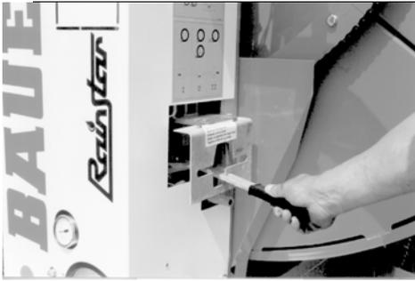
Move the gear-shift lever to the „PE-pipe pull-off“ position. A spring presses the lever up and locks it.
