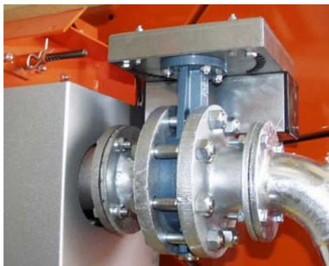
With the overpressure shut-off valve, water supply to the machine is turned off completely at the end of the irrigation run. When the valve closes, pressure rises in the supply line.
