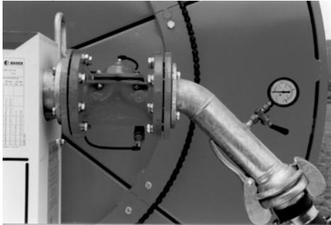
With the overpressure shut-off valve, water supply to the machine is turned off completely at the end of the irrigation run. When the valve closes, pressure rises in the supply line.
