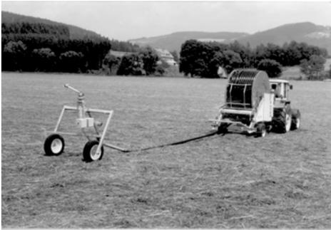
If required, you can rewind the PE-pipe also with the tractor's PTO system.
