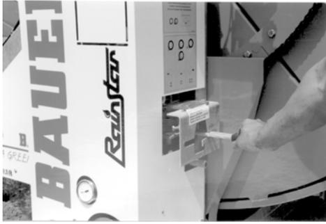
...and slacken the PE-pipe by pressing the shut-off lever downward slowly and carefully.
