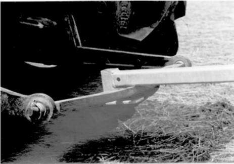
You pick up this hook with the tractor's toolbar and pull the cart across the field. For turning the pipe reel and placing the RAINSTAR in a new setting-up position, the cart must be in its end position.
