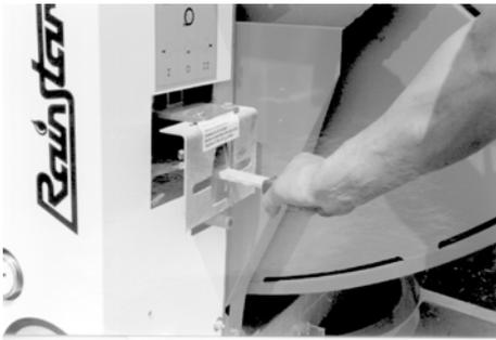
Slacken the PE-pipe by carefully pushing the gear shift lever down.
