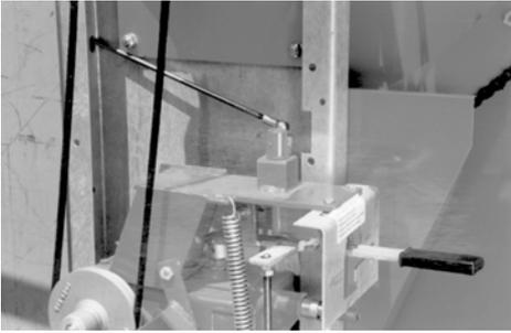
BAUER change-speed gearbox reduces the turbine speed according to the set retraction speed. The gearbox incorporates four gears. Reel drive stop at the end of the irrigation strip is ensured by disengagement of the tooth clutch.
