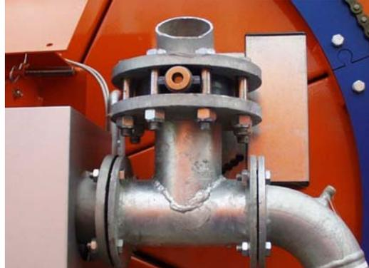
With the low pressure shut-off valve option, a diaphragm valve is opened quickly at the end of the irrigation run, releasing a big water stream into the open. This causes sudden pressure decrease in the supply line (to about half the original pressure). Through this drop in pressure a pressure switch shuts off the pumping unit and thus also the water supply.
