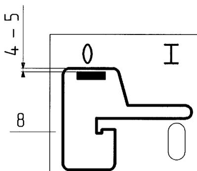
Turn the hex. nuts (6) on the threaded rod (7) apart until a spacing of 4 to 5 mm results between the shifting gate (8) and the shut-off lever (9).
