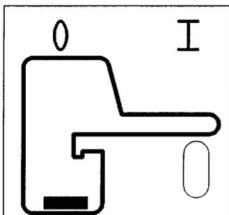
In this position the brake band must be lifted slightly off the brake disc. This prevents the brake band from sticking to the brake disc!
