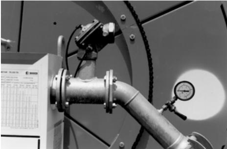
With the low pressure shut-off valve option, a diaphragm valve is opened quickly at the end of the irrigation run, releasing a big water stream into the open. This causes sudden pressure decrease in the supply line (to about half the original pressure). Through this drop in pressure a pressure switch shuts off the pumping unit and thus also the water supply.
