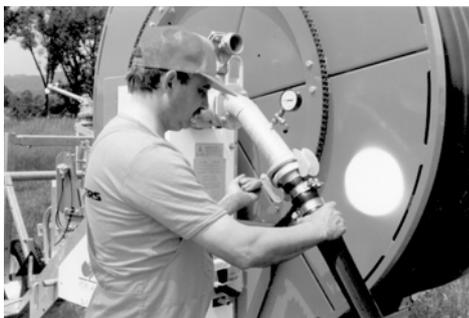
Slacken the PE-pipe by pushing down the gear shift lever carefully.
