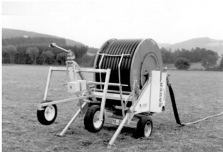
At the end of the run the cart is lifted automatically and the drive is shut off through shut-off rods.
