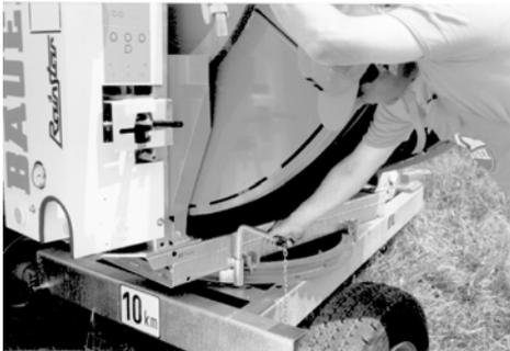
For lateral pull-off remove the lock bolt, turn the reel into the direction of the driving lane and secure it again with the lock bolt.
