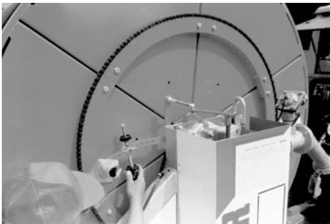
Loosen the knurled nuts that secure the adjusting lever. Set the desired retraction speed with the adjusting lever – the speed is indicated on the tachometer (optional equipment). Afterwards secure the adjusting lever again with the knurled nuts.
