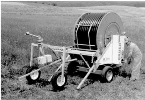
When you drive the reel with the PTO, the automatic final shut-off is inactive. Therefore you must stop the PTO in time and wind up the end of the PE-pipe with the hand wheel. This will prevent damage to cart, shut-off, gearbox, etc.
