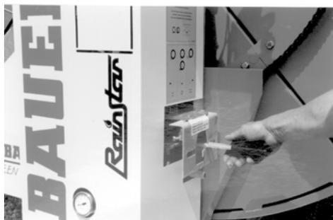
If something unforeseen happens you can interrupt pipe retraction. Pull or push the gear shift lever with your open hand from gear position I or II into the middle position. (Do not operate the lever with your hand closed, or let it go immediately). The gearbox is disengaged, 0 position. A spring presses the lever up (shut-off position) and prevents fast reversing of PE-pipe or reel.
