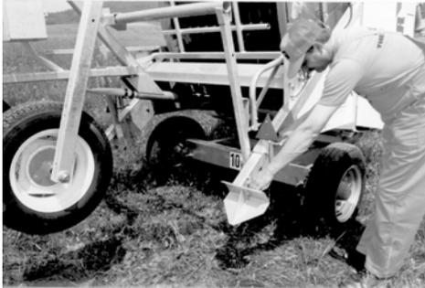
2. Move gear shift lever to the middle position and slacken the pipe by pushing the lever down slowly and carefully.
