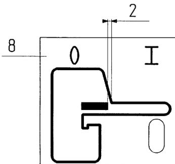
The shut-off point is reached when the PTO shaft no longer turns along. Set the shifting gate in this position according to the drawing ( 2 mm)!
