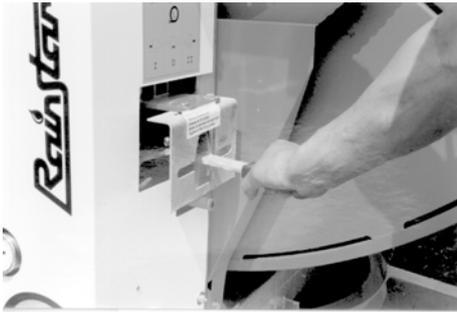
Move the gear shift lever from a gear stage to the middle position. A spring presses the gear shift lever up and prevents fast reversing of the reel and PE-pipe by means of the band brake. By pushing the gear shift lever down very slowly you release the brake and slacken the PE-pipe.
