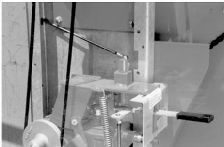
The water supply is stopped by means of the „overpressure shut-off valve“ option, or the pumping unit is shut down by the „low-pressure shut-off valve“ option in combination with a pressure switch in the supply line.
