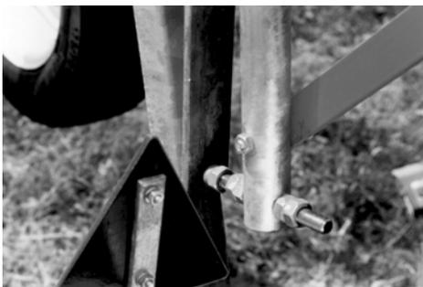
Unattended performance of the RAINSTAR is made possible by a final and safety shut-off. The final shut-off is actuated when the sprinkler cart presses against the shut-off frame, which in turn operates the gear shift lever through a system of rods. This way the drive is stopped.
