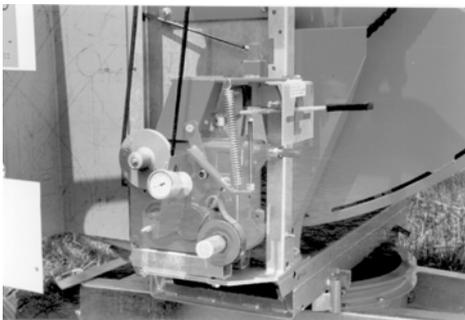
The change-speed gearbox contains gear wheels which reduce the turbine's speed accordingly. The gearbox features two speeds. Reel drive stop at the end of the irrigation strip is achieved by disengagement of the toothed clutch.
