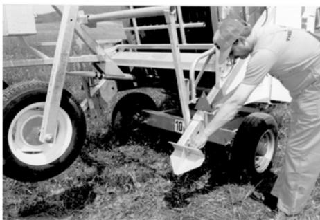
When the pipe has been fully rewound, relieve the machine supports with the hand wheel, move them into the transport position and secure them with the locking bolts.
