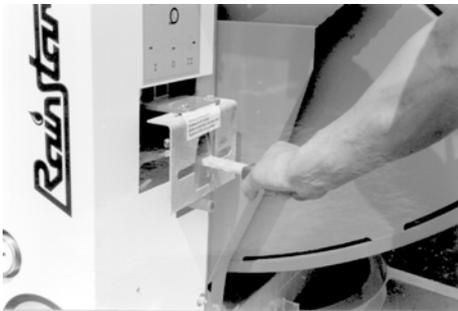
Push the gear shift lever downward carefully - the carts moves down slowly.
