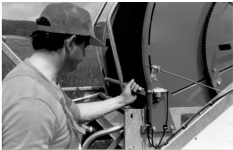
Therefore this valve can only be used in combination with an automatic pump shut-off device or in a line network supplying several machines. Before starting up with water again the hand lever must be shifted to the START position (downward) - the shut-off valve is relieved and opens.
