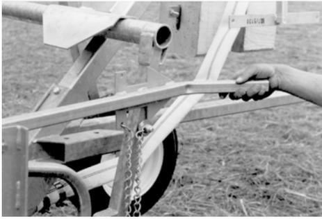
Pick up the draw-out hook with the toolbar and pull off the cart.
