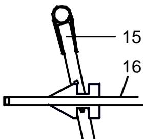
If shut-off is not actuated, proceed as follows: Hook up the cart lift bracket (15) with the locking hook (16).
