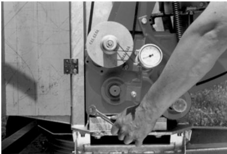
Drain screw for gear oil.
