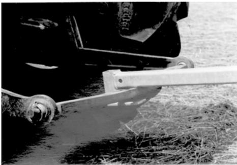
Pick up the draw-out hook with the toolbar and start pulling the cart .
